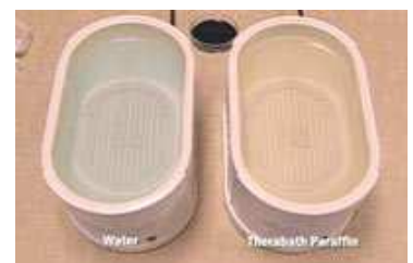
This demonstration illustrates that the contaminant (blue dye) does not disperse into the paraffin bath.
